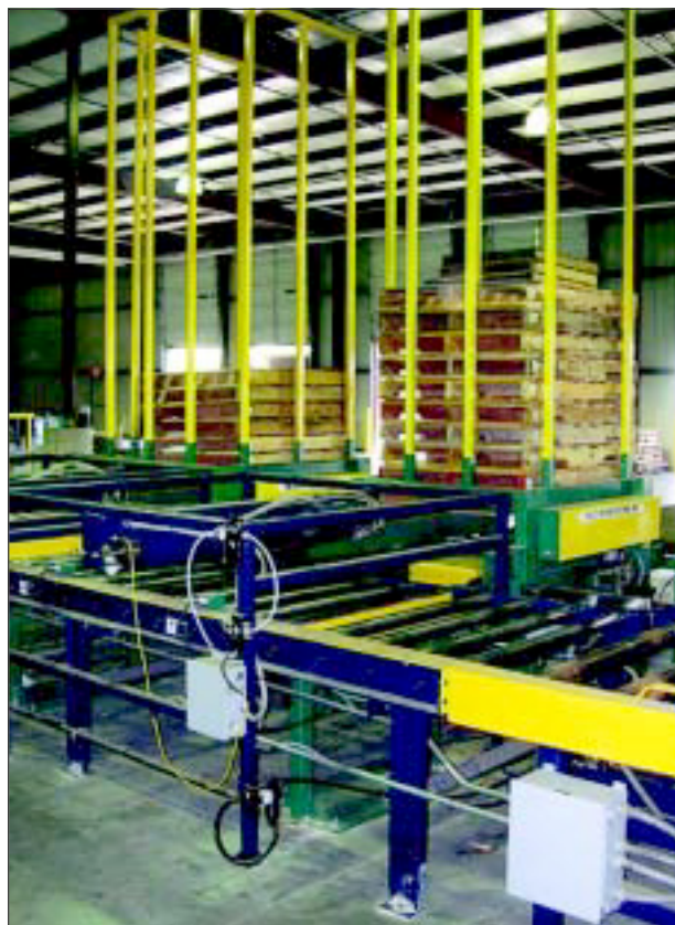
In the stacking area, a scanner reads the bar code label, and the pallet is automatically sorted and stacked by the PRS equipment.
