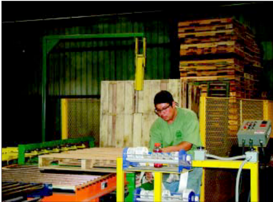
Each repair worker attaches a bar code to the pallet identifying the employee, work station, and grade of the pallet.
