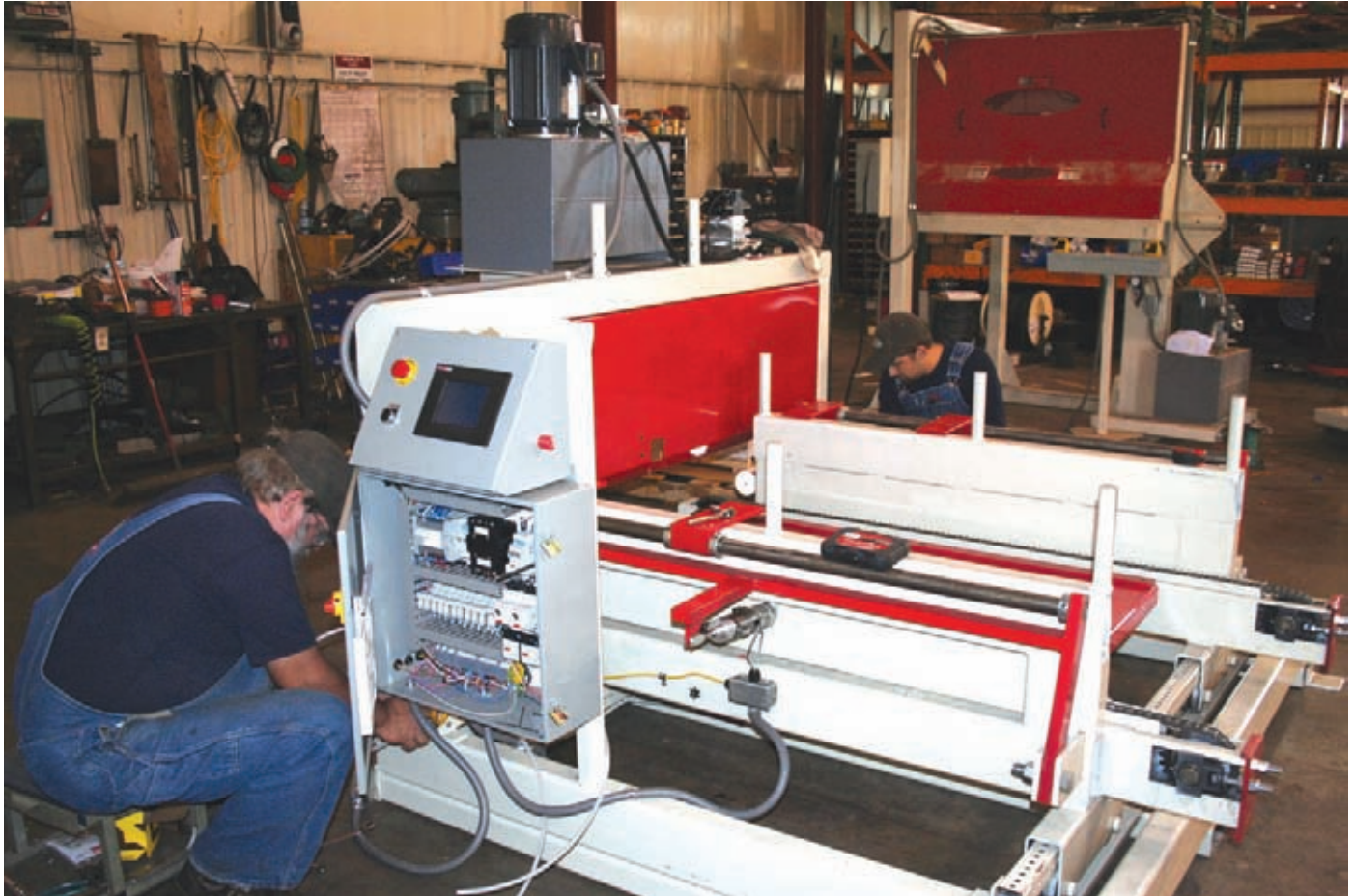
Pallet dispenser under construction. Pallet dispensing is a growing trend in the materials handling function.
