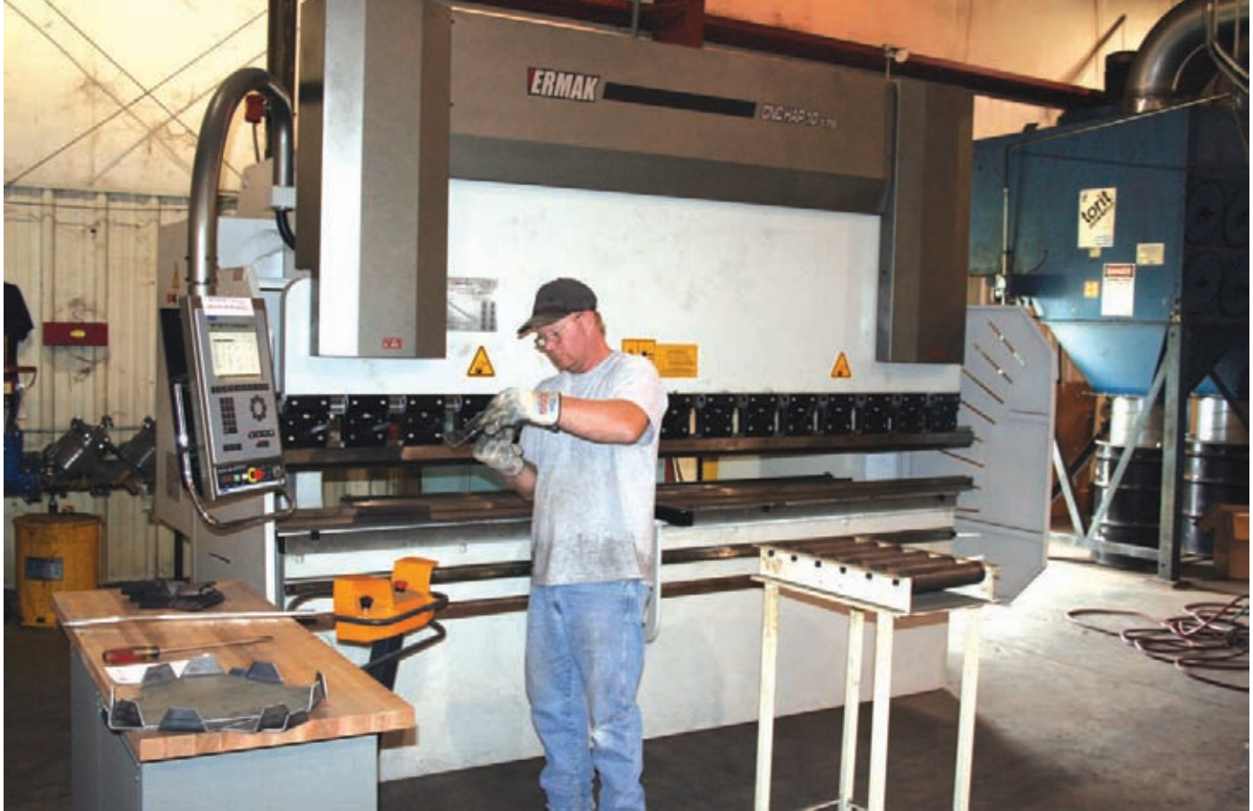
This press brake is an example of the kind of manufacturing machinery needed in an efficient manufacturing company.
